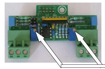
Calibration screws: Compare readings with an accurate digital thermometer
