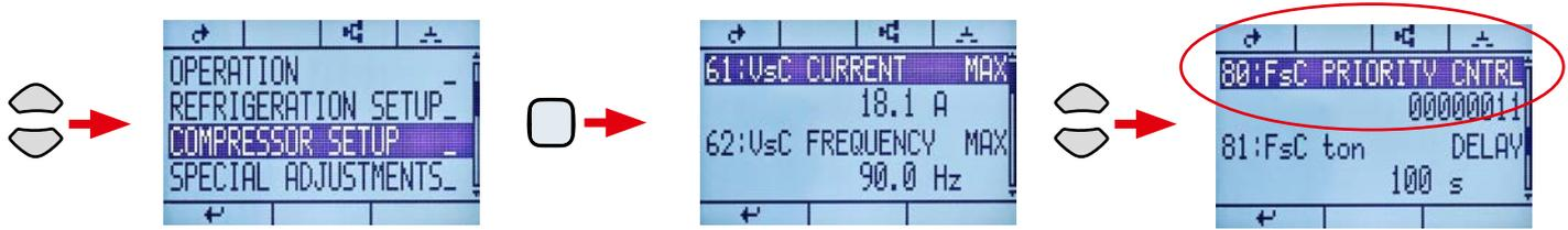
Press key "OK" to enter the parameter input window. Skip to next digit with arrow keys "Left" and "Right". Change value of digit with arrow keys "Up" and "Down". Every digit "1" corresponds to a FsC in the rack system, as shown below. The value of parameter 80 entered has to be confirmed with key "OK".
