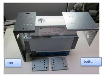
Position the IP40 housing parts as shown on the left (black cover on top side and back side of bottom cover below) and fix with the screws of step 1.
