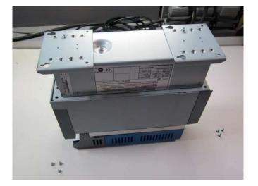
Remove the screws holding the two mounting plates. Keep the screws for further installation.
