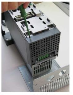
Fix the cable mounting bracket using the two screws to the left and right of the power terminal and motor cable connections.
