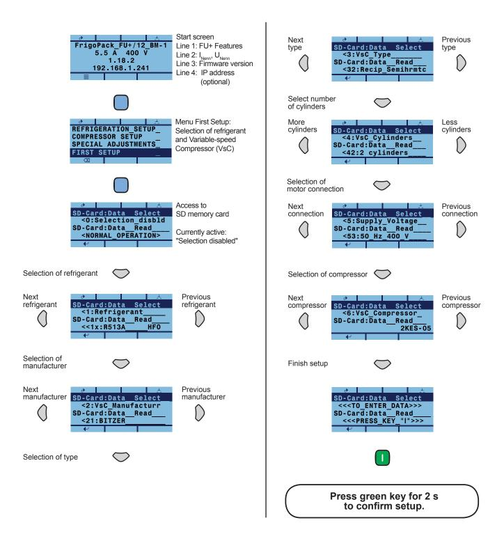
After pressing the green key for 2 s menu "First Setup" can be left with the "Back" key.
